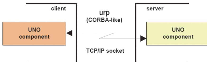
Figure 4: Communication between UNO components [Flat05].
